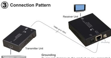
To prevent damage to the product or any connected devices, and to improve audio/video signal quality, it is recommended to ensure that the extender systems are properly grounded.
